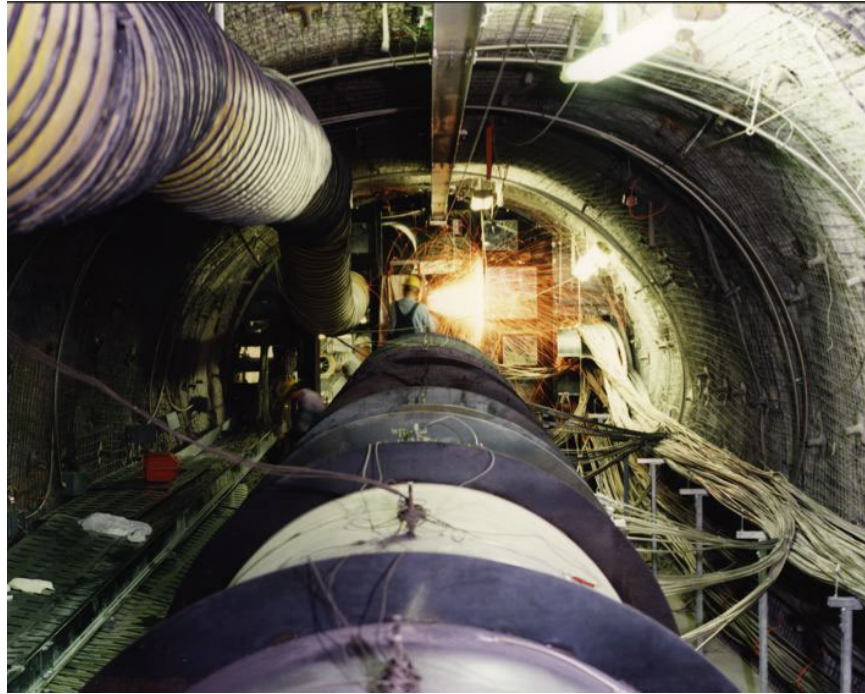
Figure 6 View of the Electric Heaters (center) in the Drift during Set-up for the Heated Drift Experiment
