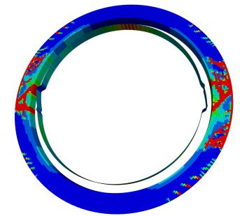
A new concrete constitutive model and non-linear structural elements (ground support) have been added to FLAC3D 9. Here you can see a section through a shaft lined with concrete which is yielding and an inner steel liner that is buckling.
