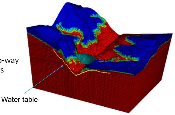
Dam model with impounded water saturation contours shown
