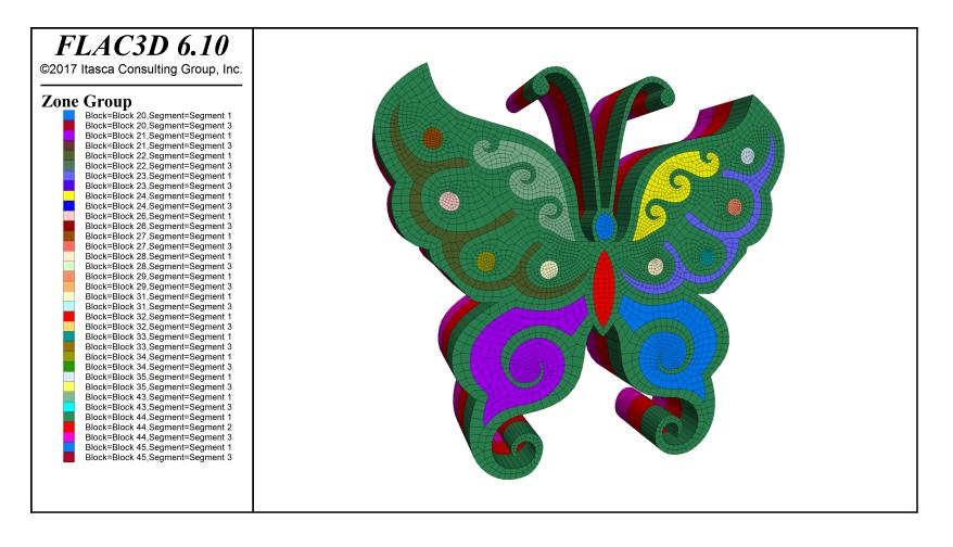
Finite volume formulation does not require a regular grid – unstructured meshes are possible
